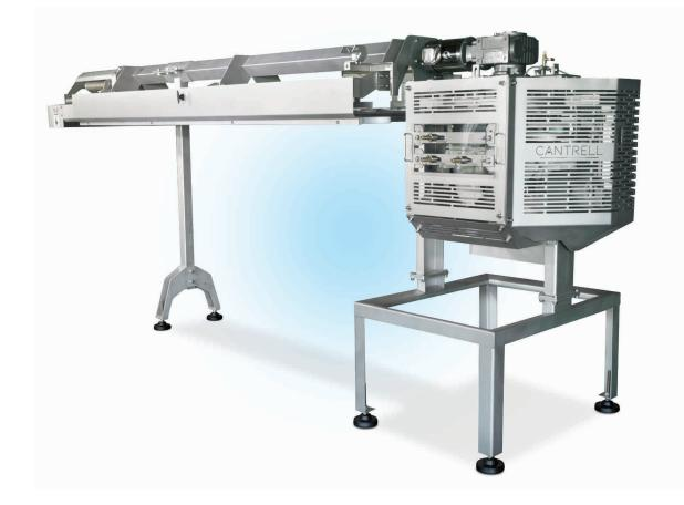
**The Cantrell Wing Segmenter** offers flexibility, accuracy and ease of use for your operation. The machine is capable of processing up to **180 wings per minute** on a processing line or as a standalone application. The Wing Segmenter properly orients the wing at any line speed for accuracy on each individual cut.
