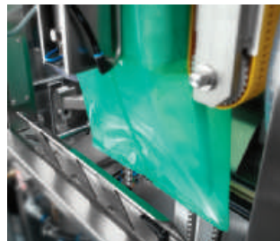
Zero Reject Sealing System guarantees airtight seal even if contaminants are present in the seal area
