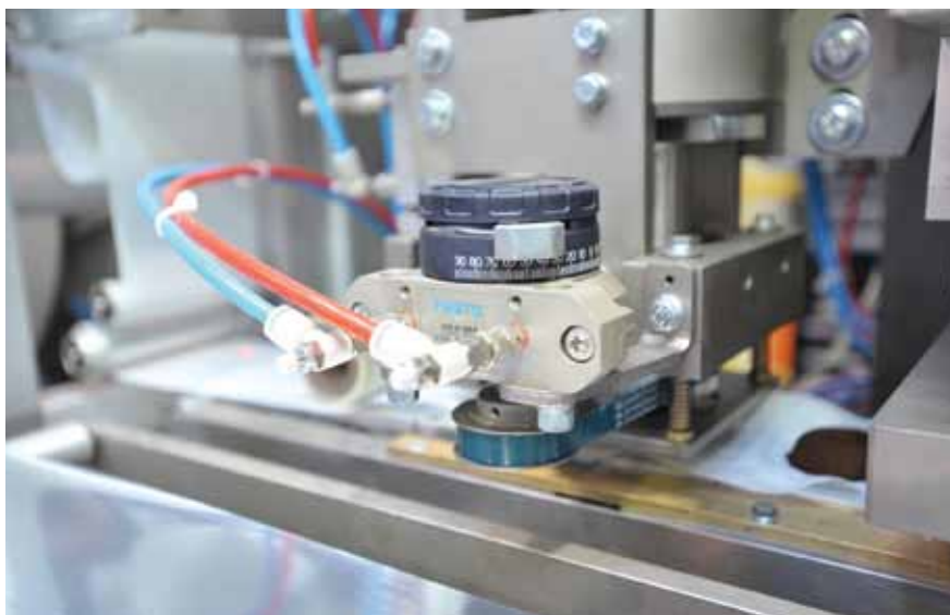
A Festo semi-rotary 0-180 degree air cylinder mounted to the bottom of an auger filler on the OPEM Kikka tamps and twists to release the coffee grounds for even dispensing of the product onto the pod's filter paper.
