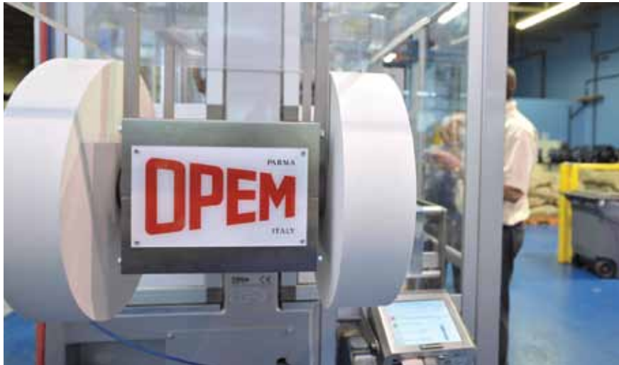
The Muldoon's Own OPEM Kikka coffee pod-forming machine uses filter paper manufactured by the Glatfelter company.
